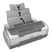
2. Place the hooks on the back of the matte sheet support over the paper support extension, then slide it all the way down.
